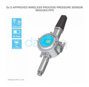
WS433EX-PPS is the Sub-GHz Integrated Process Pressure Sensor with Exd approval for installation in Zone 1, Zone 2, or Safe Zone. It has different measurements, such as Gage/Absolute/Sealed Gage, range -1 .. + 1000 bar, high accuracy, and stability. With an Ultra-low-power design and smart firmware, the sensor can last up to 10 years with a single C battery (depends on configuration). The sensor will connect to a Wireless Coordinator WS433-CL or iConnector with the built-in wireless coordinator.
