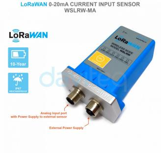
WSLRW-MA is the LoRaWAN wireless sensor with one channel to measure 0-20mA DC current from Process instruments like Pressure transmitter, Temperature transmitter, Level transmitter, Flow meters, Analyzers... at very low voltage drop. With Ultra-low-power design and smart firmware allow the sensor can last up to 10 years with 2 x AA batteries (depends on configuration). The sensor will transmit data in the kilo-meters distance to LoRaWAN gateway, any brand on the market.
