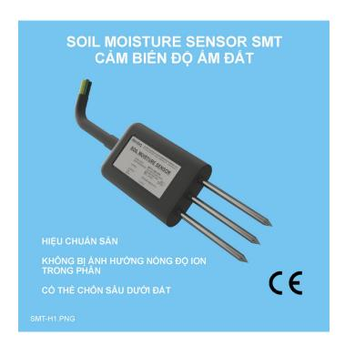
SMT is a soil moisture, soil temperature and soil EC. Utilize advanced technology, Frequency Domain Reflectometry to deliver high accuracy and stable measurement of Soil Moisture, not affected by Fertilizer contents and Temperature like the simple Capacitance Moisture Sensor on the marker. Sensor output is RS485 / modbusRTU easily connected to any control and monitoring system. Typical applications are: intelligent irrigation systems, greenhouses, soil condition check...
