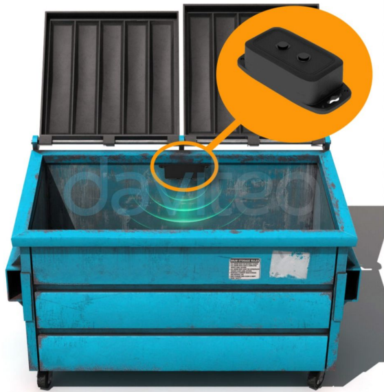
MOUNTING ULA SENSOR ON LARGE TRASH BIN
