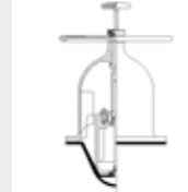
Non-rising handwheel with indicator DN200 - DN300 8" - 12"
