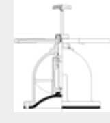
Non-rising handwheel with indicator DN200 - DN350 8" - 14"
