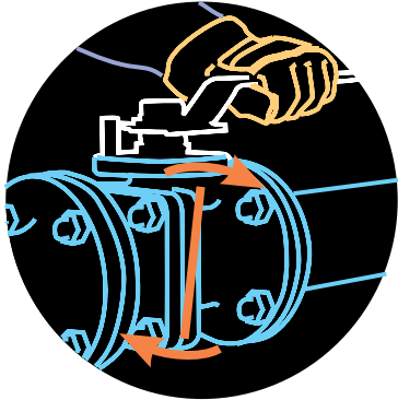
Heavy manual operation
