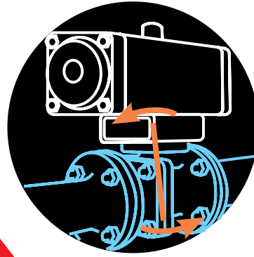
Actuation loads and misalignment
