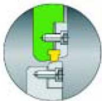
Fig.6 Rubber seal(Replacement seat)
